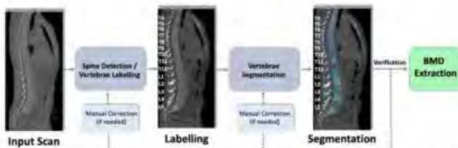
Fig. 1: The automated spine processing and vBMD extraction pipeline is used to localize, label, and segment the vertebrae.
